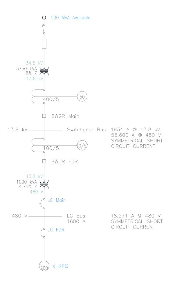
Short-circuit and load currents. Short-circuit and load currents must be determined and included on the appropriate time-current coordination curves or entered into the computer plotting program.
